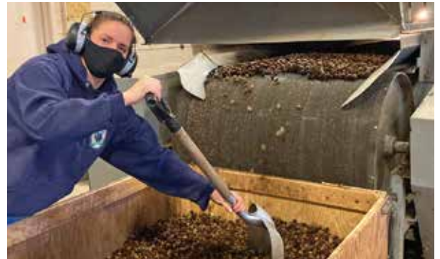
Black spruce is running through an "extractor," which is a large oven that heats the cones and allows them to open and release seeds. This is mostly used for serotinous cones (jack pine), but sometimes black spruce cones are opened this way as well. This is what the end of the oven run process looks like. Cones are collected in a large hinged box. Cones are shoveled to disperse them evenly throughout the box.
