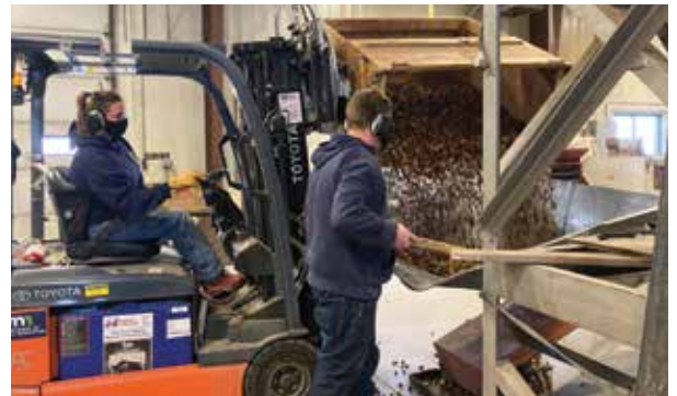
The open cones that just came out of the oven are dumped into a large hopper attached to a conveyor. The cones travel up the conveyor and into a large tumbler, then work their way through the tumbler and release seeds into hoppers under the machine. The cones come out of the far side.
