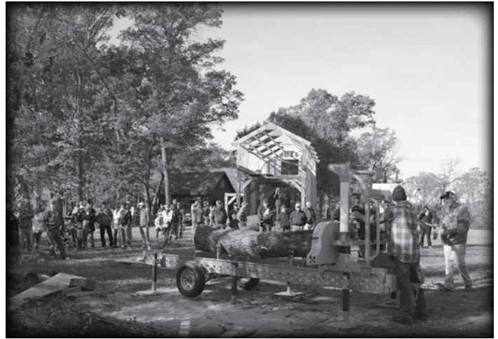
A portable sawmill and a new building starting from home-sawed lumber.
