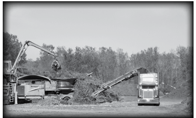
Logs and branches are reduced to chips in the wood yard.
