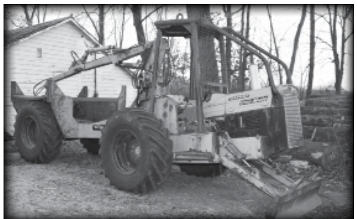
Below: The only major piece of equipment Dave uses in his woods is this Iron Mule, made in Upper Michigan in the 1970s. "I like to keep all my logs free of dirt and other debris. With this Iron Mule, I can wind my way up to a felled tree and pick up the logs without ever skidding them."
